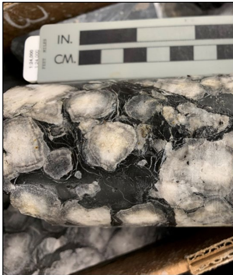
Figure 7.10 Coarse dolomite alteration in the JL LCZ in SC19-251 at 533.6 m depth
