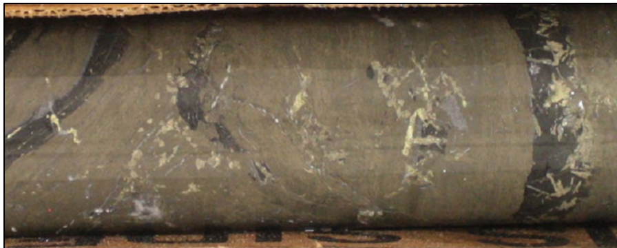
Figure 7.17 Interbedded pyrite and siltstone from the northern part of the JL UCZ. Coarse chalcopyrite and crystalline pyrite have replaced tabular barite crystals. Coarse chalcopyrite also forms veinlets cross-cutting bedding. Core diameter = 63.5 mm
