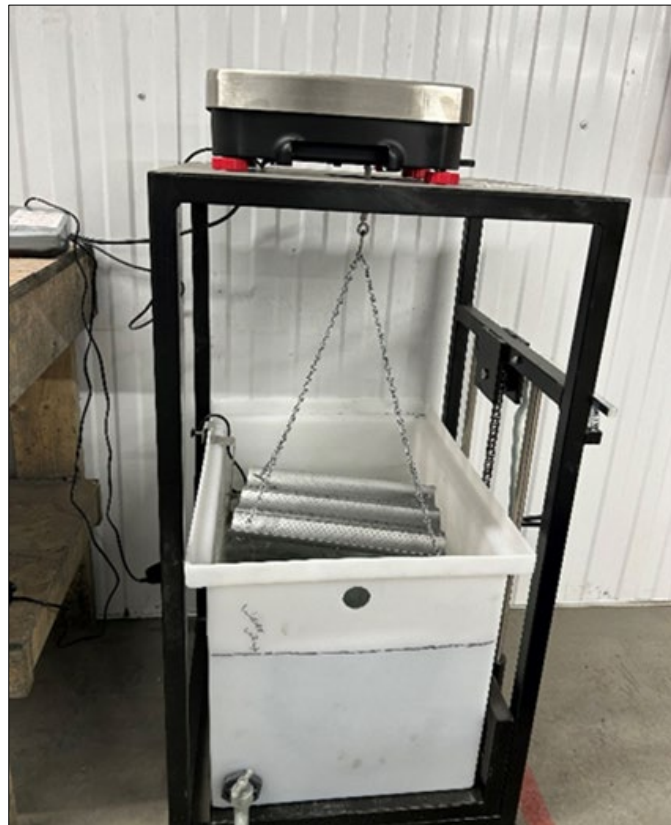
Figure 11.2 Specific Gravity Station in SFA Core Logging Facility
