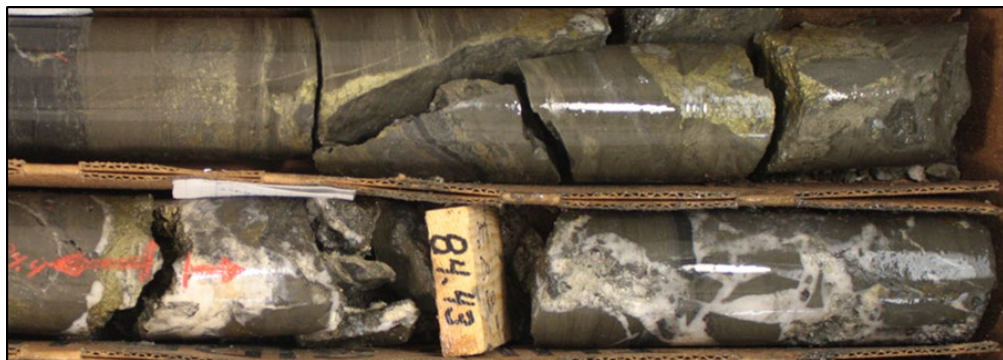
Figure 7.16 Coarse chalcopyrite that is synchronous with hydraulic brecciation, fracturing and quartz-carbonate veins. Core diameter = 63.5 mm
