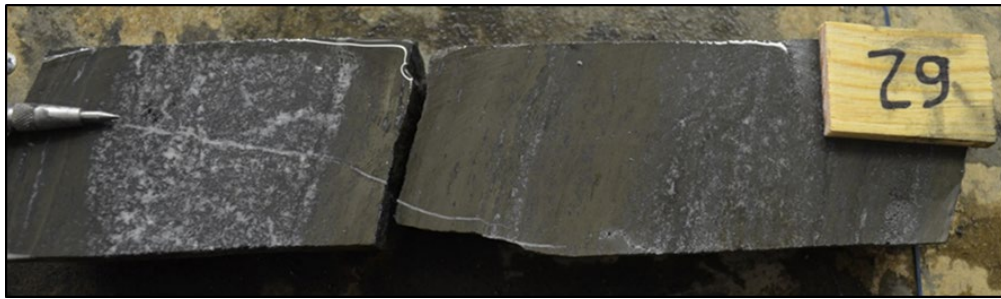
Figure 7.13 Photograph of JL USZ bedded pyrite sulfide containing net texture with light colored infilling
