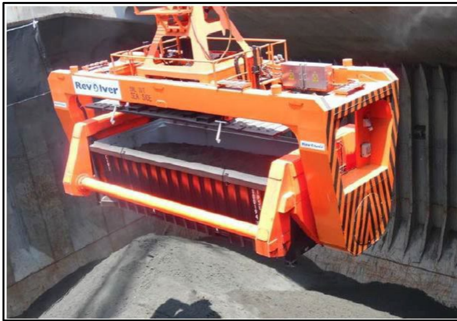
Figure 19.3 Photograph of Ram Tipper
