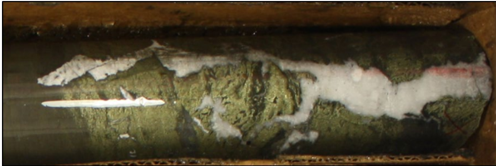
Figure 7.15 Coarse chalcopyrite, cross-cut by quartz-carbonate veins in JL UCZ. Core diameter = 63.5 mm
