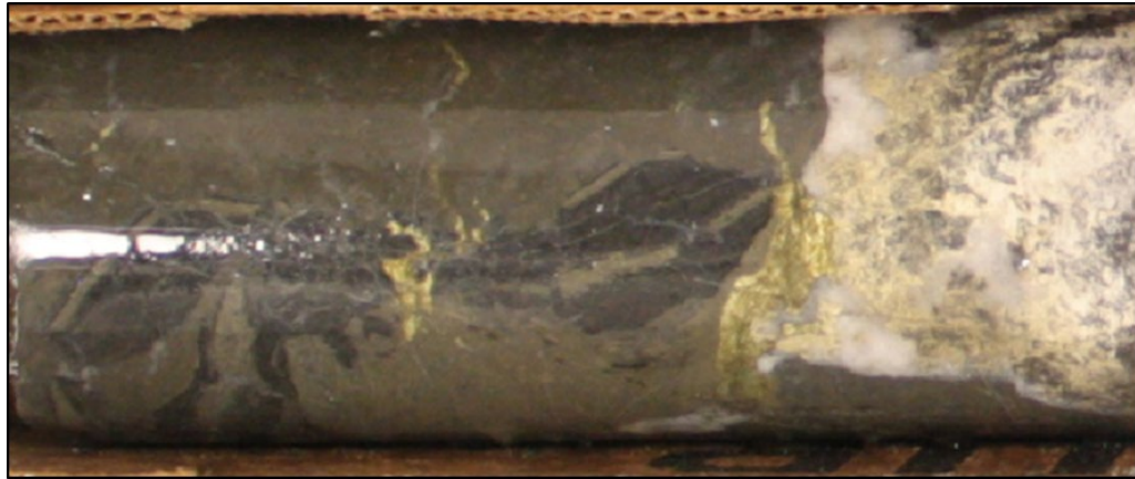
Figure 7.18 Coarse chalcopyrite both synchronous and post-dating quartz-carbonate veining in the northern part of the JL UCZ. Core diameter = 63.5 mm
