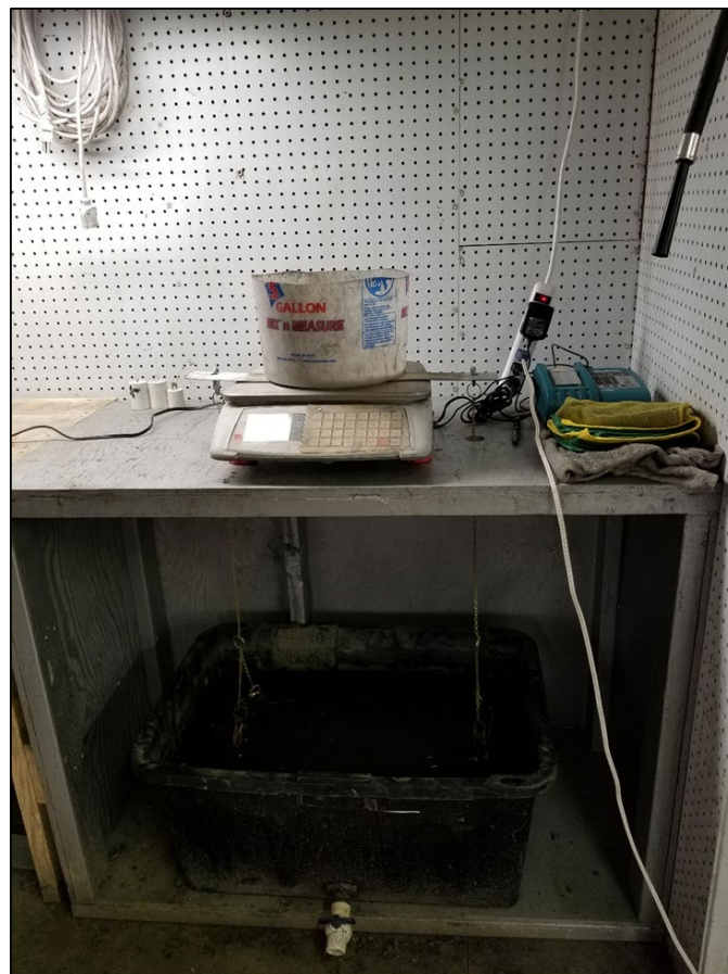
Figure 11.1 Specific Gravity Testing Apparatus at the Sandfire Resources America Inc Logging Facility 2018-2022
