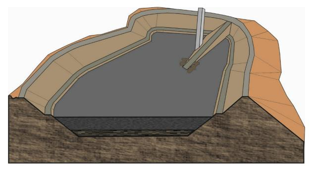
Using the estimated surface areas of the paste and the waste rock, we estimate mass-load inputs by scaling to the appropriate humidity cell test of pasted tailings, ultimately predicting water quality in the sump. The model further evaluates the predicted sump water quality with a PHREEQC geochemical model, allowing precipitation of supersaturated phases and sorption to ferrihydrite surfaces if ferrihydrite is supersaturated.
