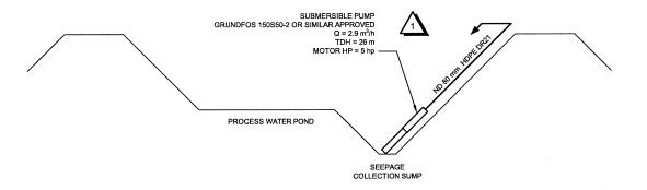
PROCESS WATER POND SEEPAGE COLLECTION AND RECYCLE SYSTEM
