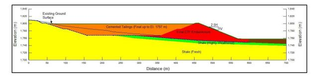
Figure 6.1 CTF Typical Cross-Section
