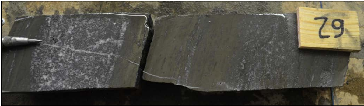
Figure 7-13: Photograph of USZ Bedded Pyrite Massive Sulphide Containing Light Colored Atoll-Textured Units
