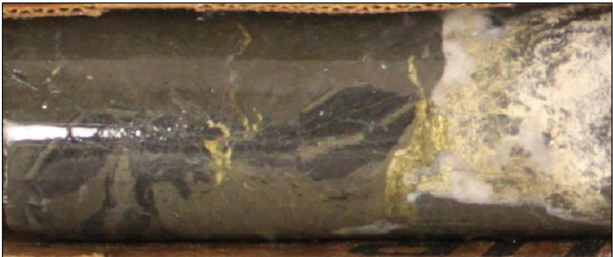
Figure 7-22: Interbedded Pyrite with Siltstone Layers from the Northern Part of the UCZ
