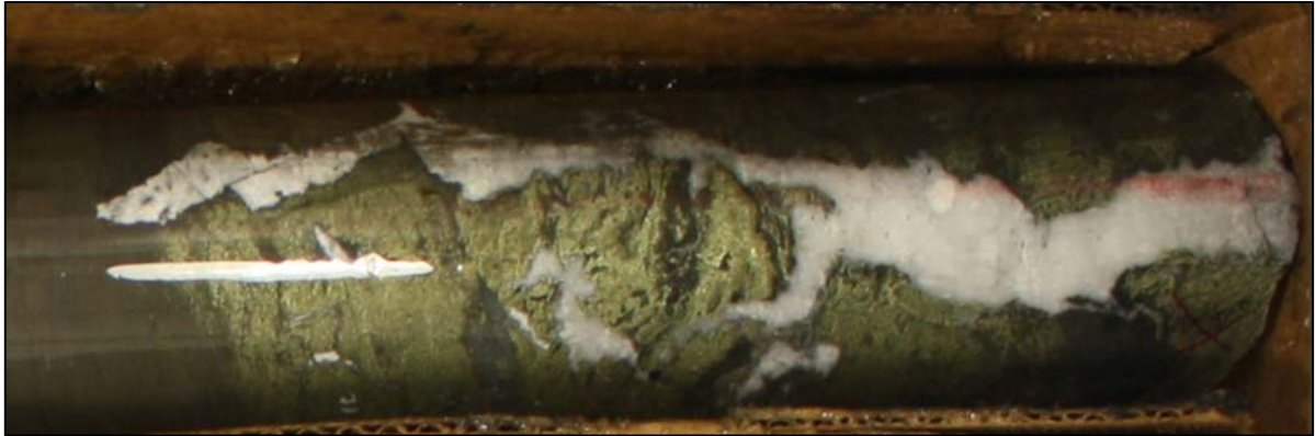
Figure 7-20: Coarse Chalcopyrite, Cross-Cut by Quartz-Carbonate Veins
