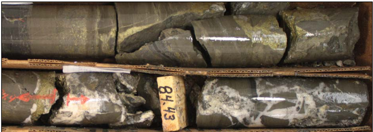
Figure 7-20: Coarse Chalcopyrite, Cross-Cut by Quartz-Carbonate Veins
