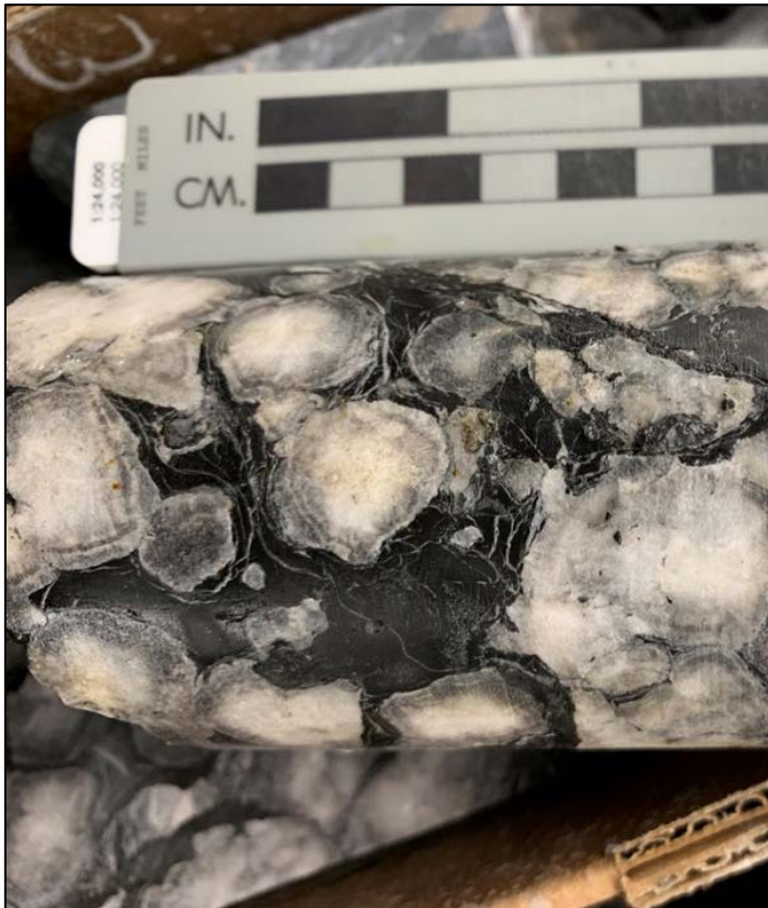
Figure 7-10: Coarse Dolomite Alteration in the LCZ in SC19-251 at 533.6 M Depth
