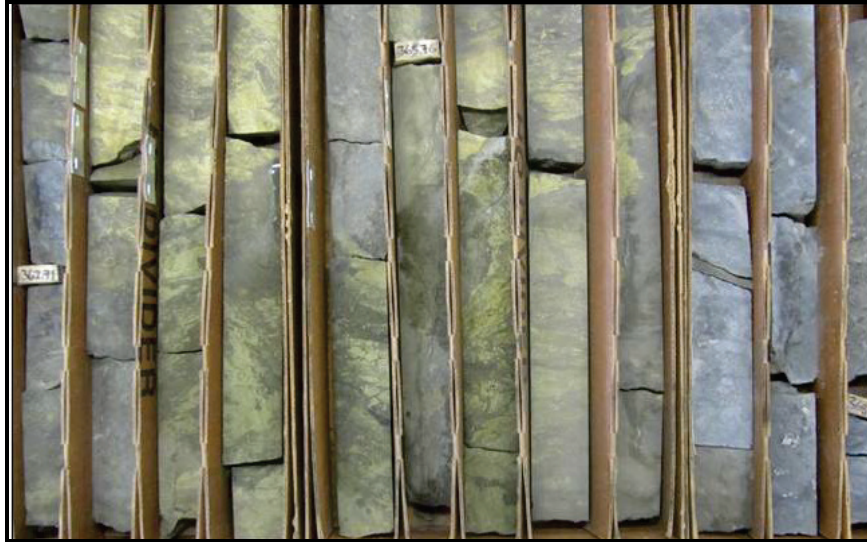
Figure 7.11 High-grade LZ Mineralization – SC11-048
