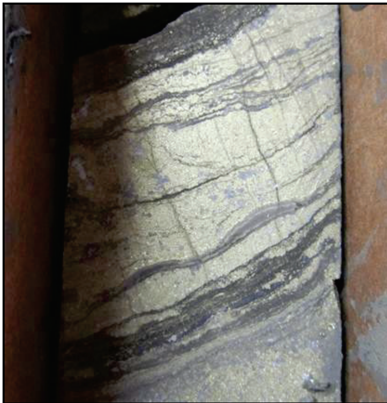
Figure 7.10 Finely Bedded LSZ Mineralization – SC10-004
