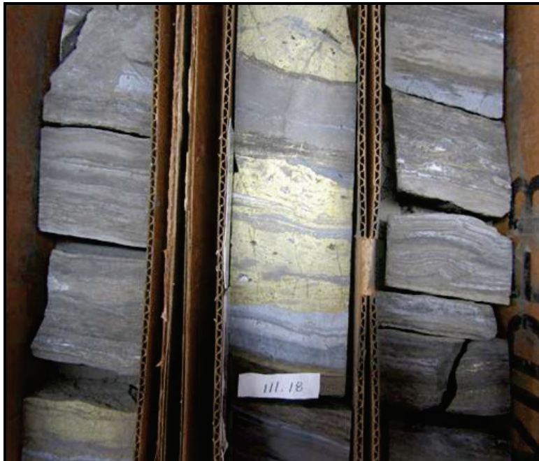
Figure 7.8 Bedded Massive Sulphide Mineralization – SC10-004
