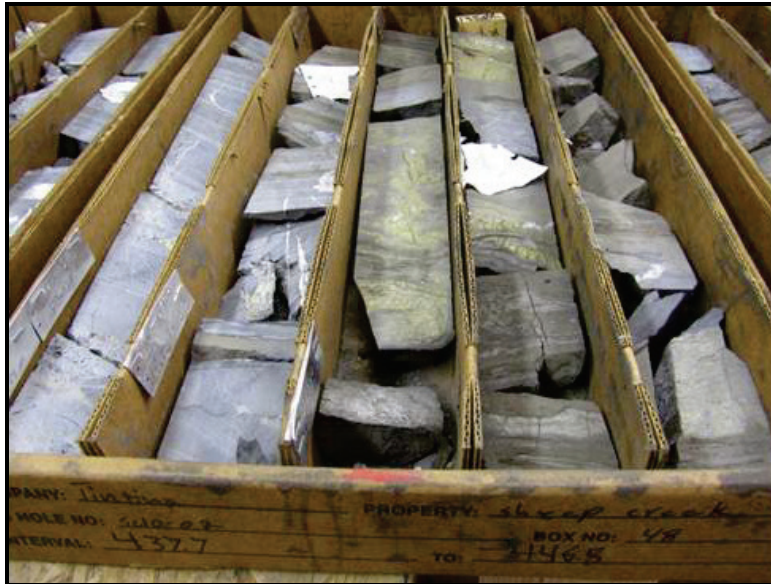
Figure 7.7 Fine-grained Chalcopyrite Mineralization – SC10-002
