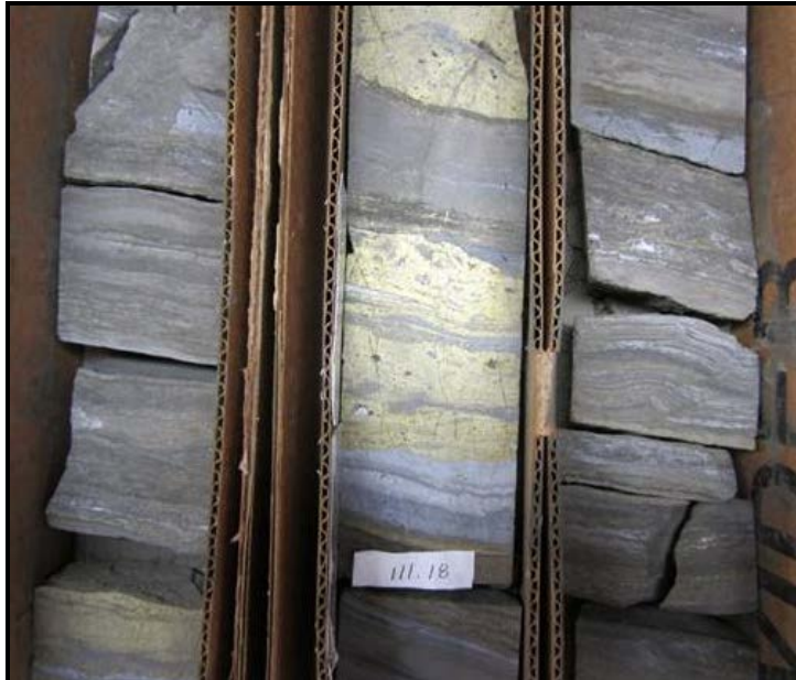
Figure 7.9 Bedded Massive Sulphide Mineralization – SC10-004
