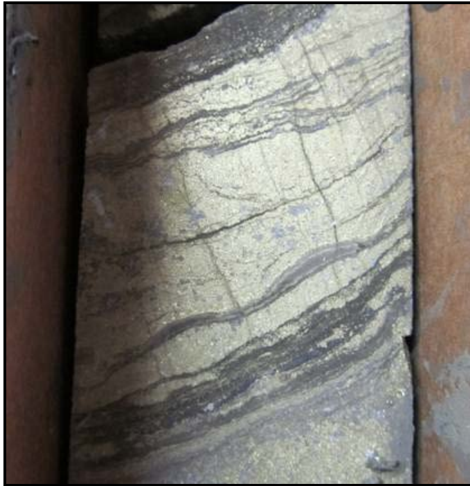
Figure 7.11 Finely Bedded LZ Mineralization – SC10-004
