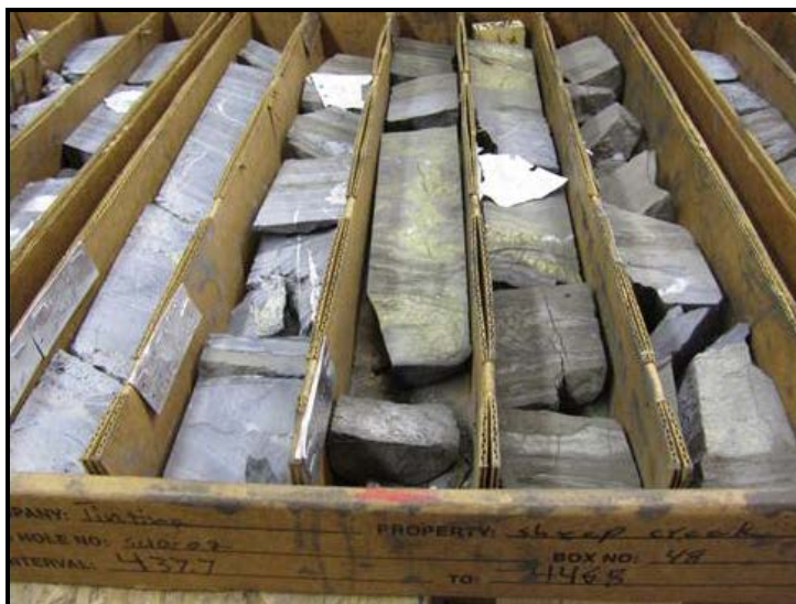
Figure 7.8 Fine-grained Chalcopyrite Mineralization – SC10-002
